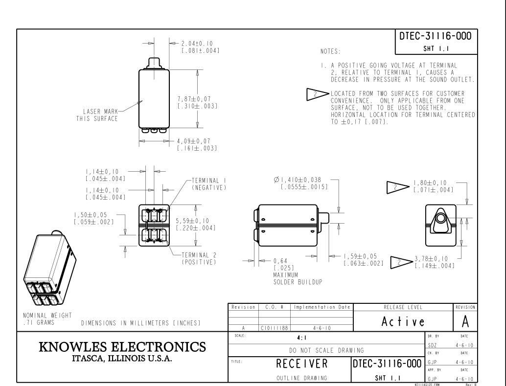
THE DTEC-31116-000 IS A PAIR OF BALANCED ARMATURE RECEIVERS INTENDED FOR USE IN BTE HEARING AIDS. IT HAS A LOW DCR TO IMPEDANCE RATIO, HAS THE CENTER TERMINAL CONNECTED TO CASE AND IS THE SAME SIZE AS AN EF RECEIVER
